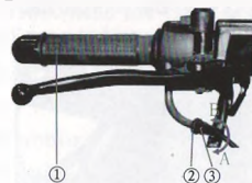
① Throttle grip ② Locknut ③ Adjusting bolt
